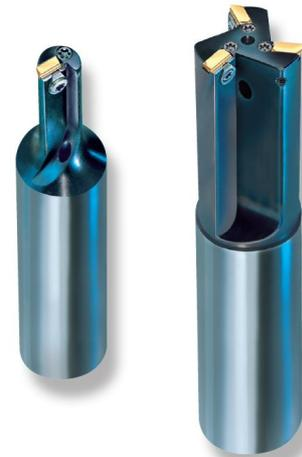
The large chip flutes in combination with embedded clamping elements guarantee an excellent chip evacuation. The clamping element has to be slightly released only in order to change the insert. However, the clamping element itself remains securely connected to the holder.
