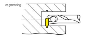
Our mini-boring bars are also perfectly suitable for every kind of form recesses. In customer specific requirements the operational possibilities of our standard boring bars can on request beenormously increased by means of special form inserts.
