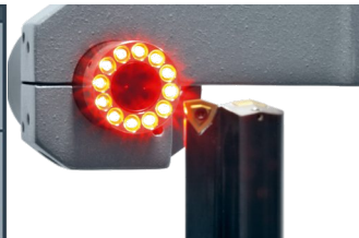
Cutting edge inspection
