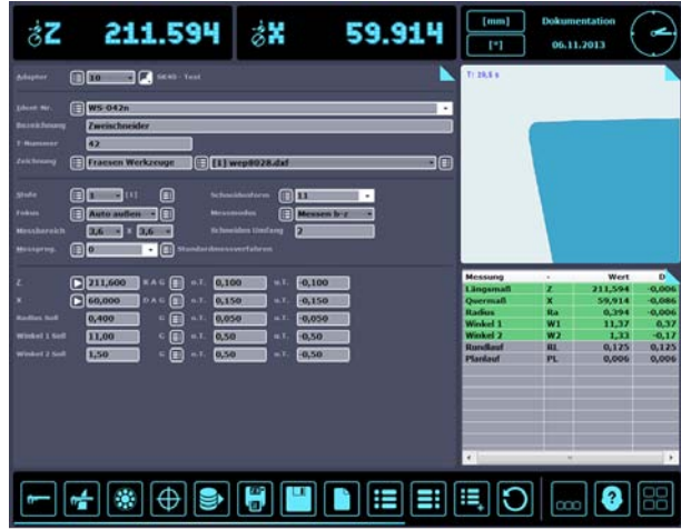
Measuring Program 0: Default measuring in transmitted light All measurements are automatically carried out with the selected edge shape.
