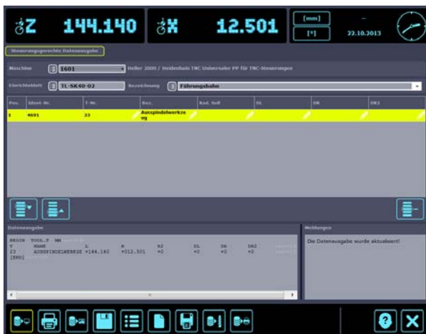
Data Output incl. Format Generator, the actual data of the measured tools are displayed control-specifically on the monitor for data output
