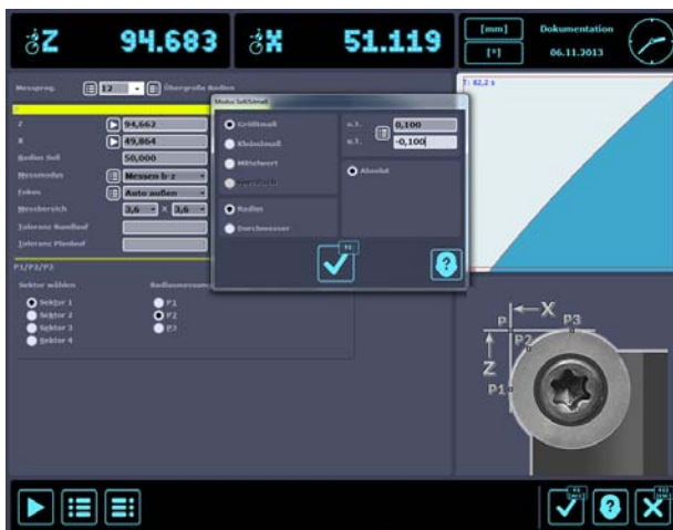
Measuring Program 12: Oversize Radii This measuring program covers large radii along with the tolerances assigned to them.
