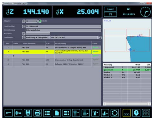
Tool Management, This function allows you to integrate your ZOLLER presetter/measuring machine with myTouch operating technology »pilot 2 mT« into ZOLLER TMS Tool Management Solutions. This way you can manage all your tools in a single, central database.
