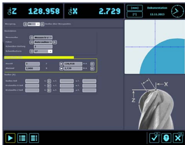
Measuring Program 31: Theoretical circle center by measuring points By defining a number of measuring points on the cutting edge you can use this program for concave/convex tools to find out their theoretical circle center and radii.
