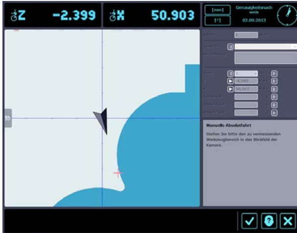
Navigation system »compass« for a quick and comfortable axis adjustment for nominal positioning
