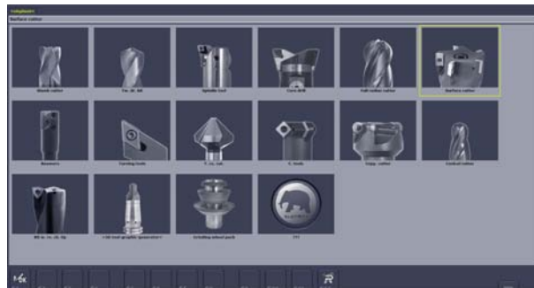
Step 1: Select type of tool from the image catalog of standard tools.
