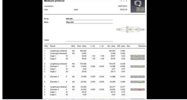
Documentation, Saves measured results and provides protocols or an analysis for all variants of measured values.
