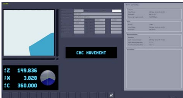
CNC-drive of axes, Automatic, operator-independent and safe positioning of the axes into the target position. The operator can stop the axes manually at any time - any risk of injury is precluded!
