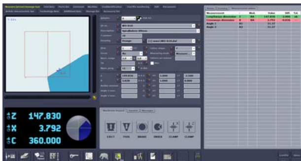
Tolerance check automatically checks the dimensional correctness of the measured parameters and provides these to the operator in a clear and unmistakable manner.
