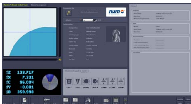
Interface num, Interface for tool grinding machines with NUMROTOplus software as of software release 2.6.2. for the fully automated measurement of tools without requiring programming effort.
