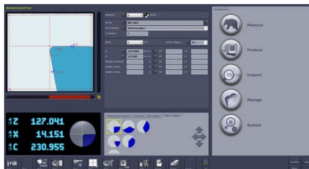
Automatic cutter shape detection, The cutting geometries are recognized automatically and only suitable measuring routines are offered.
