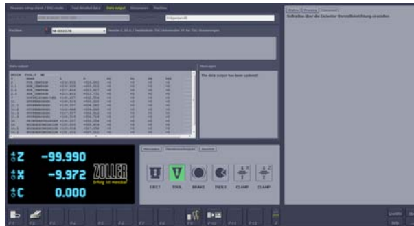
System-guided measuring programs with photo-realistic input dialog. For example, largest cutting edge on milling heads, concentricity and run-out, theoretical point on drills, etc.
